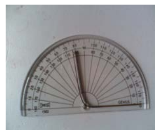
Figure 4 Shows the SMA strip after recovery.
